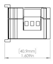
DIMENSIONS ARE IN INCHES TOLERANCES: (UNLESS NOTED) 3 PLACE DECIMAL = ±0.005 2 PLACE DECIMAL = ±0.015 1 PLACE DECIMAL = ±0.050 DIMENSIONS IN INCHES DRAWING NOT TO SCALE
