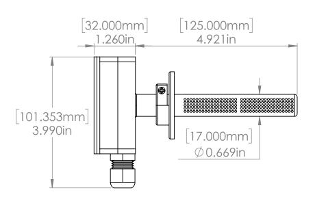
DIMENSIONS ARE IN INCHES TOLERANCES: (UNLESS NOTED) 3 PLACE DECIMAL = ±0.005 2 PLACE DECIMAL = ±0.015 1 PLACE DECIMAL = ±0.050 DIMENSIONS IN INCHES DRAWING NOT TO SCALE
