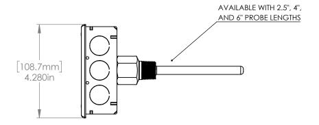
DIMENSIONS ARE IN INCHES TOLERANCES: (UNLESS NOTED) 3 PLACE DECIMAL = ±0.005 2 PLACE DECIMAL = ±0.015 1 PLACE DECIMAL = ±0.050 DIMENSIONS IN INCHES
