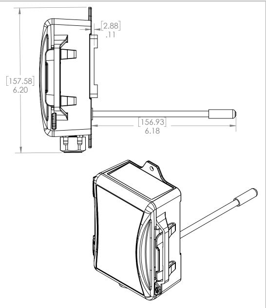
DIMENSIONS ARE IN INCHES TOLERANCES: (UNLESS NOTED) 3 PLACE DECIMAL = ±0.005 2 PLACE DECIMAL = ±0.015 1 PLACE DECIMAL = ±0.050 DIMENSIONS IN INCHES DRAWING NOT TO SCALE
