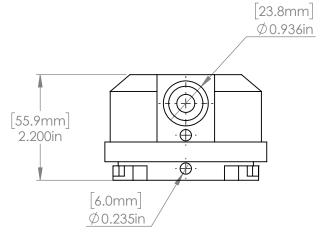
DIMENSIONS ARE IN INCHES TOLERANCES: (UNLESS NOTED) 3 PLACE DECIMAL = ±0.005 2 PLACE DECIMAL = ±0.015 1 PLACE DECIMAL = ±0.050 DIMENSIONS IN INCHES
